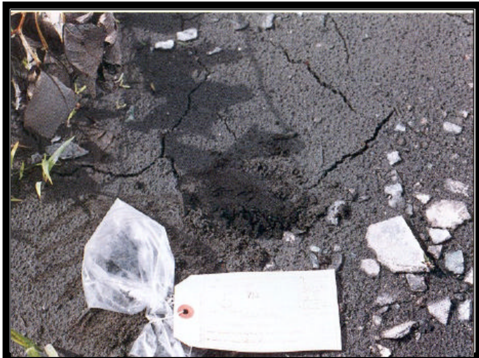
FIGURE 16. Very dark or black “soil” that turns light gray when dry. Fragments in lower right. All are asbestos.
