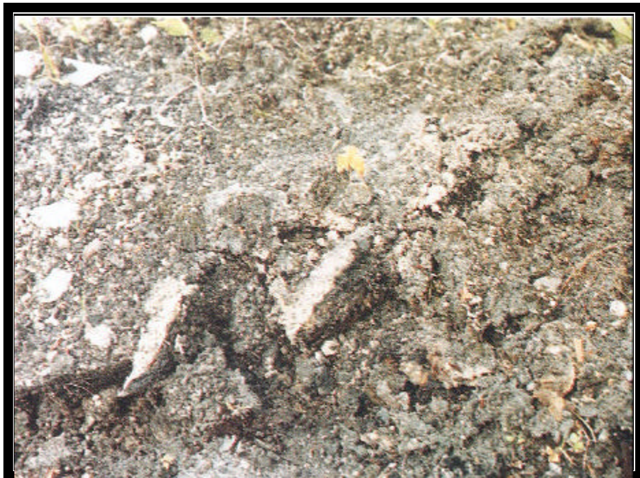
FIGURE 8. Gray or green deposits that have an unnatural soil appearance, usually void of grass, should be suspect.
