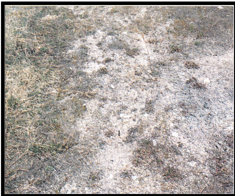
FIGURE 4. Areas of no or poor vegetation growth, with gray or colored areas of soft material which looks different than natural soil, should be suspect.
