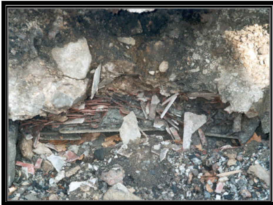
FIGURE 19. Red and gray sheet waste and plate waste, mixed with black baghouse waste (near top of photo).
