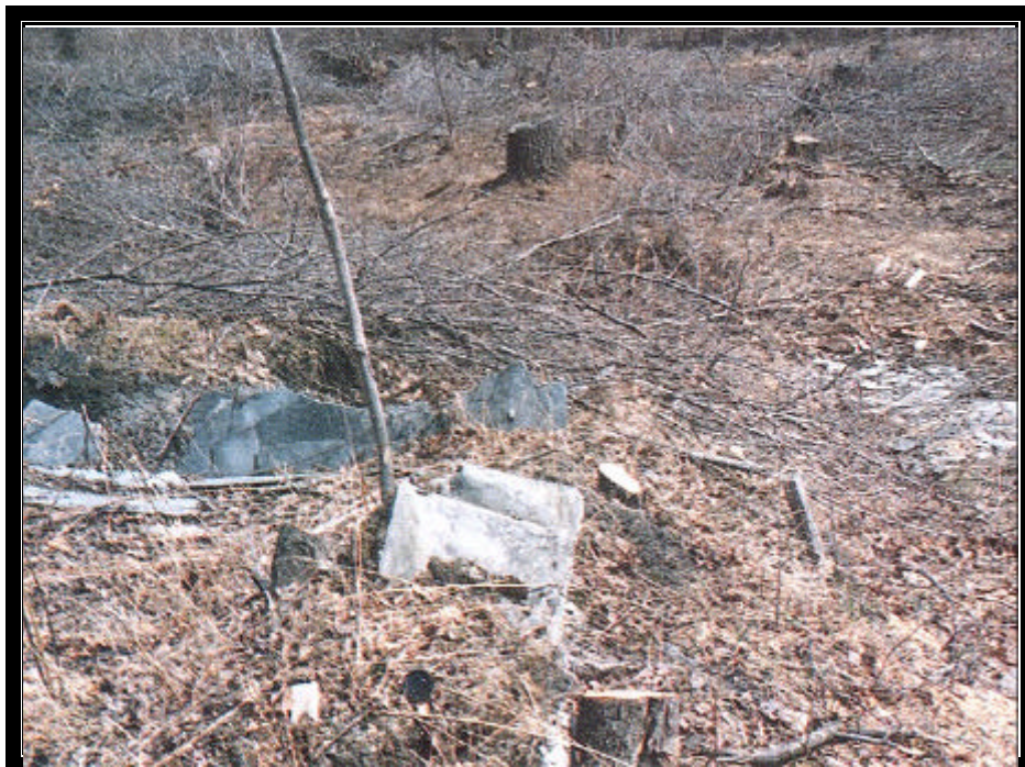
FIGURE 6. Piles or pieces of gray or colored sheets, usually 1/4" to 1/2" thick, either alone or with soft “soil,” may possibly be asbestos.
