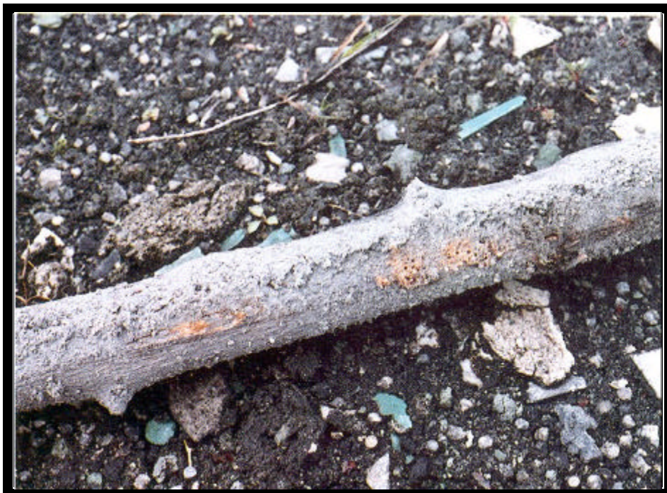
FIGURE 14. Light gray dust on black, damp soil or lighter dry soil. Note presence of green fragments and light balls. All are asbestos.
