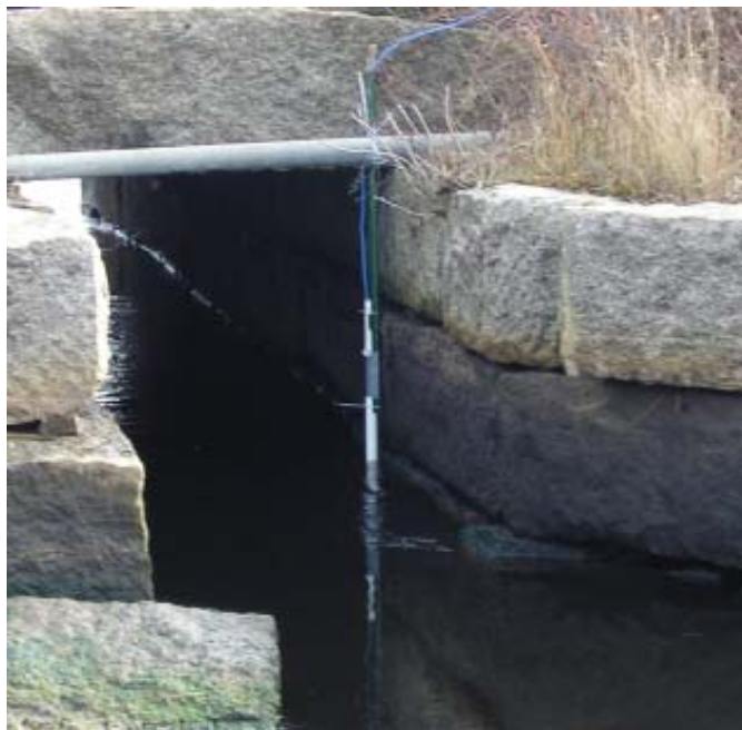
Figure 7-4: Photograph of an instrument housing that contains a temporary, continuous monitoring river gage (Source: MMI).
