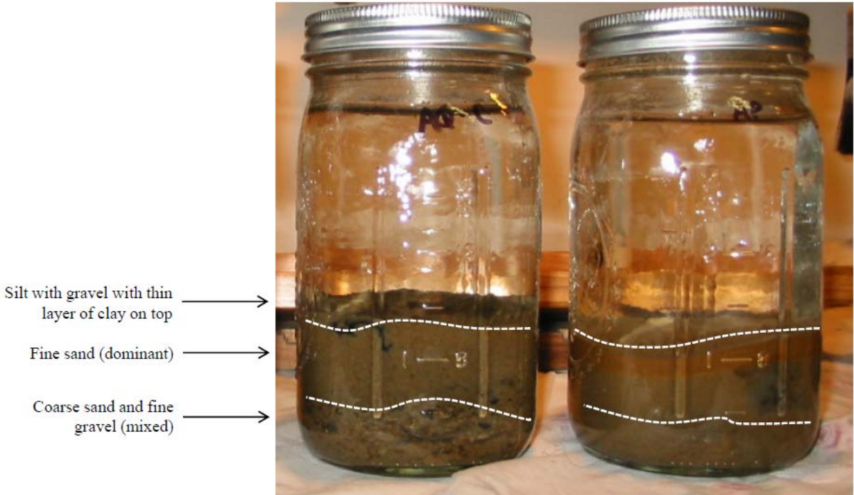
FIGURE IV-3: Jar Test to Estimate Dominant Particle Size
