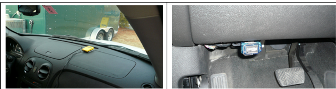
MMU – GPS positioning sensor (left) and car chip (right)
