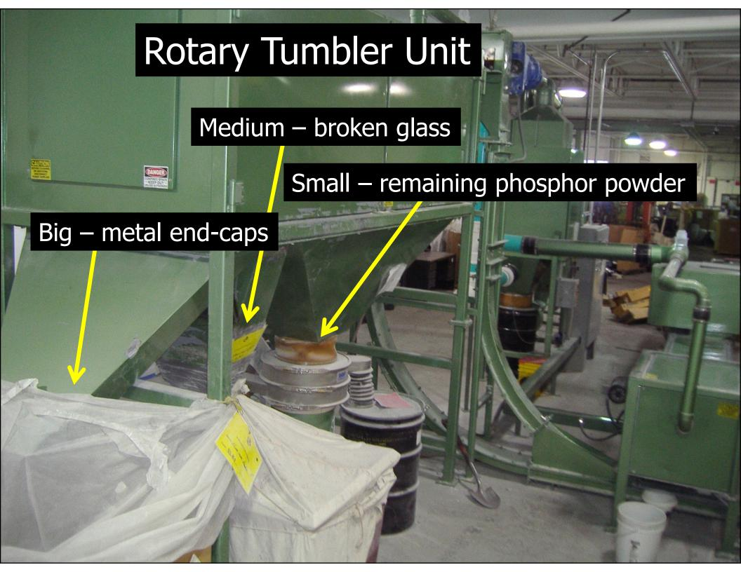
The broken glass is sent to a facility that uses it in aggregate
