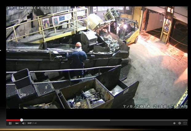
Lithium Ion Battery Entering Lead Battery Recycling Stream
