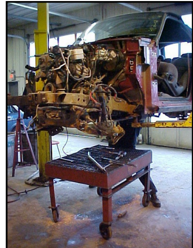
Dismantle vehicles over a concrete surface and use drain tables to fully drain parts
