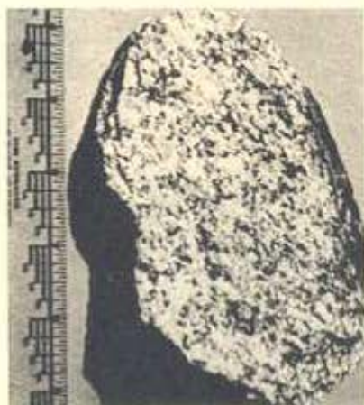
FIGURE 4. BICKFORD GRANITE Shows typical hypidiomorphic granular texture.
