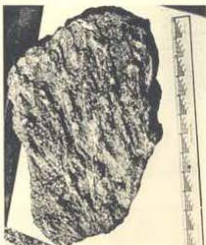
FIGURE 2. COARSE ROUGH PSEUDO-ANDALUSITE SCHIST Shows large pseudo-andalusite crystals similar to Figure 2 of Plate 5.
